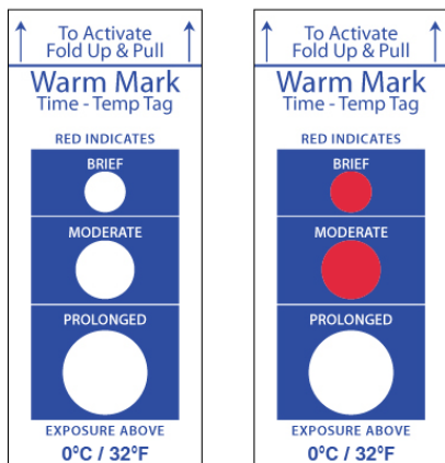
Figure 3. Temperature Indicator Tag (right) Each dry ice shipment includes a temperature tag designed to indicate exposure above 0°C. If the shipment stays below the target temperature, the windows will remain white.
